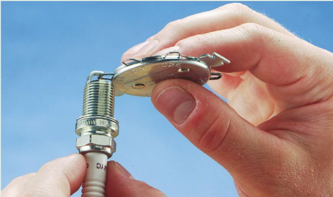
Spark plug misses under load—For more information, go to page 41
